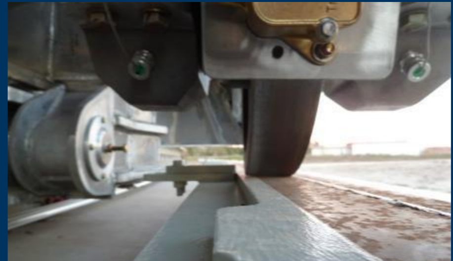
Virtually Frictionless Passive Flat Steel Wheels on Flat Steel Running Surface
