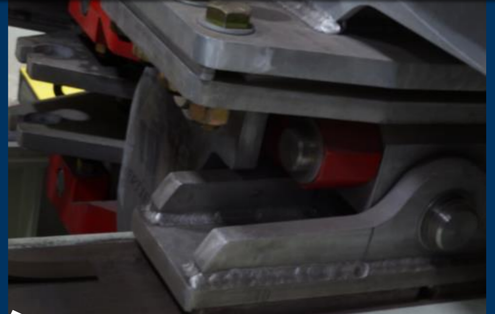
2 Sets of Hydraulic Brakes Applied to 1" Thick Steel Plate
